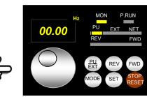
2. Turn Dial to desired Speed. (60 Hz is equal to Full Speed of Motor)
