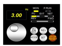
6 Push the SET Button. This stores the change you have just made. The display will now flash between the P number and the new setting.
